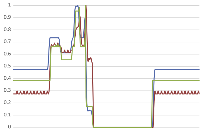
Fig. 2. Profile of the normalized backscattering values along the red lines in Fig. 1; SARViz (blue), RaySAR with incoherent summation (red), and CohRaS ® using only one scatterer per cell and incoherent summation (green). (For interpretation of the references to color in this figure legend, the reader is referred to the web version of this article.).
