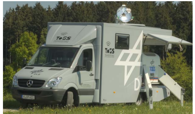
Figure 4: Transportable Optical Ground Station (TOGS)
