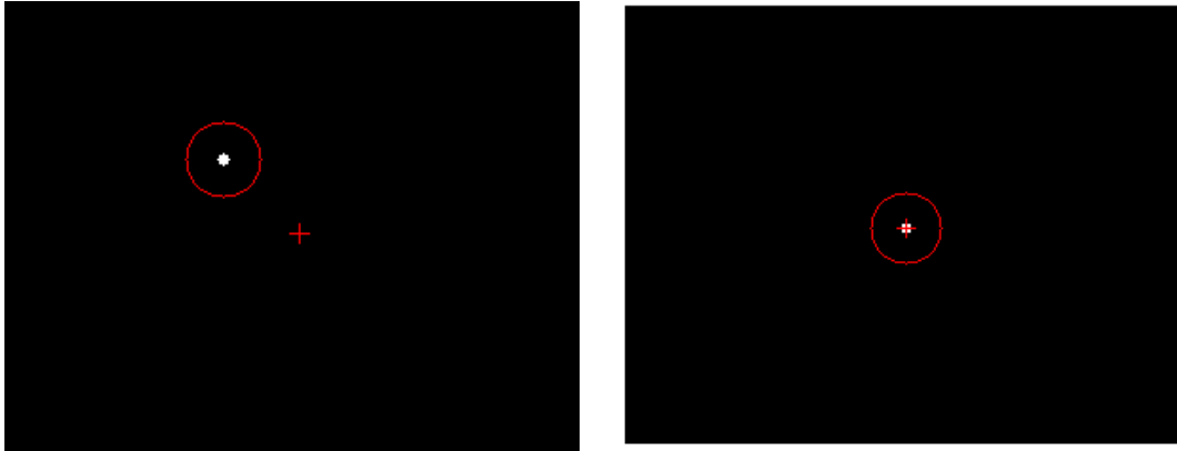
Figure 4. Tracking camera simulated image frame showing the effect of optical tracking. Left: open-loop tracking mode, Right: closed-loop/optical tracking mode. Red cross in the picture shows the spot target position and white spot is the simulated laser spot seen in the tracking camera.
