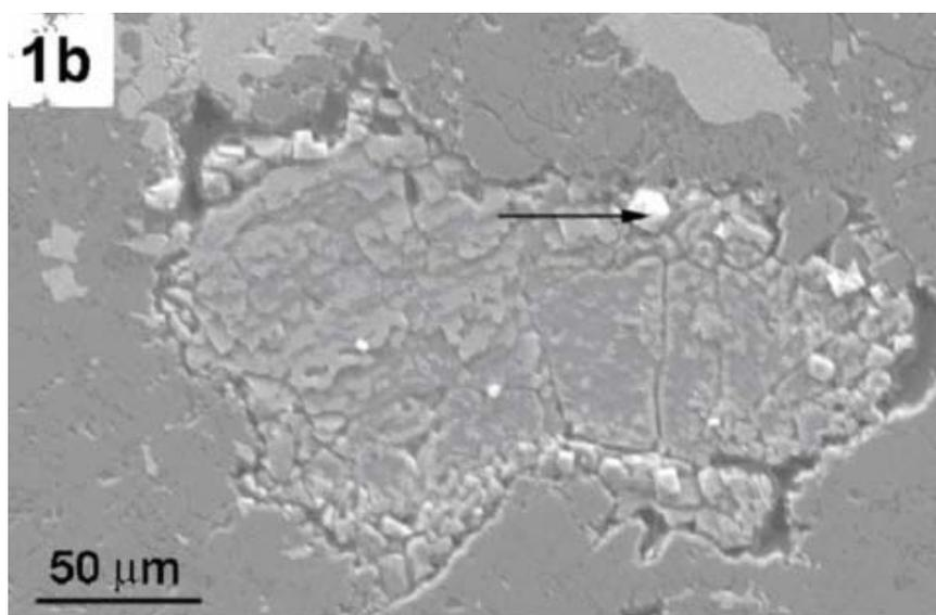
Fig.1b. Halite in Zag. There is some recrystallisation of the halite (e.g. arrowed), some of which - as around the lower margin - may be strain-induced. Secondary electron image, 20 kv.
