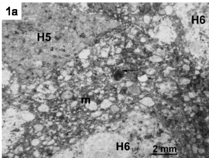
Fig.1a. Halite grain on the surface of Zag breccia. The arrow points to top margin of the halite grain showing that it has been partly fractured. H3-4 matrix (m) with visible chondrules and H5 and H6 clasts are seen. The Zag halite grains do not show evidence in the form of being part of veins or association with other low temperature mineral assemblages for crystallisation in-situ but instead appear to be clastic.
