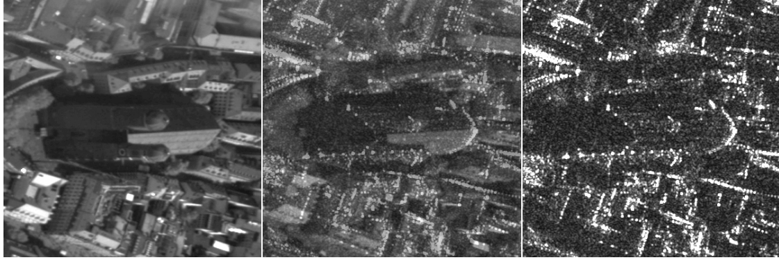
Figure 6. Zoom of Munich center - Frauenkirche – in optical VW-1 image (left), transparent overlay of optical and radar image (middle) and radar TS-X image (right) using the proposed satellite formation.
