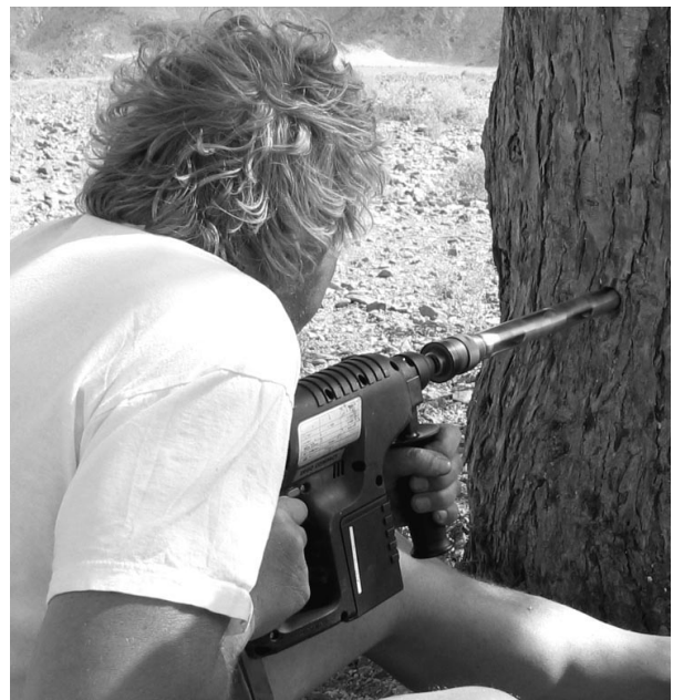
Figure 5: Sampling tree cores. To avoid destructive sampling of stem cross sections, sampling for both ^{14}\text{C} measurement and wood anatomy was based on increment coring. Due to logistic constraints a battery operated, solar-chargeable field setup was developed, including special steel corers designed to withstand the high torque.
