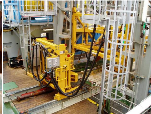
Figure 7. Skidding system for equipment handling (Source: Island Offshore Subsea, 2013)
