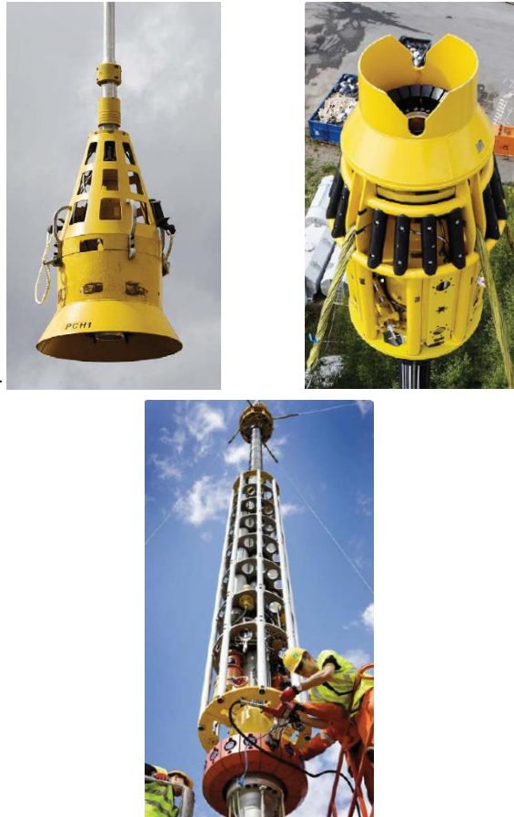
Figure 10. Upper left is the PCH, upper right is the ULP, and bottom is Lubricator Tubular (Source: FMC Technologies)
