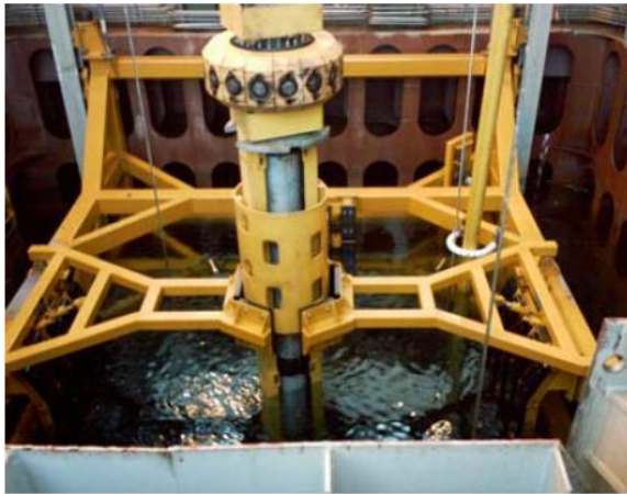
Figure 6. Lower Cursor Frame during entering the moonpool (Jøssang, Friedberg, Buset, & Gramstad, 2008)
