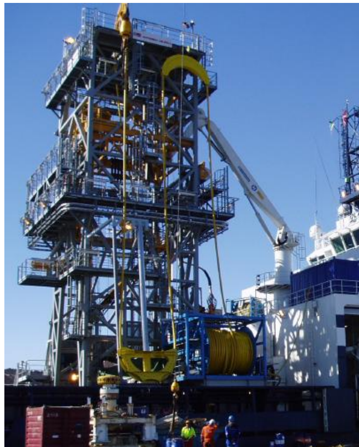
Figure 8. Heave compensation system, control umbilical, and reel installed on MHT (Mathiassen, Munkerud, & Skeels, 2008)
