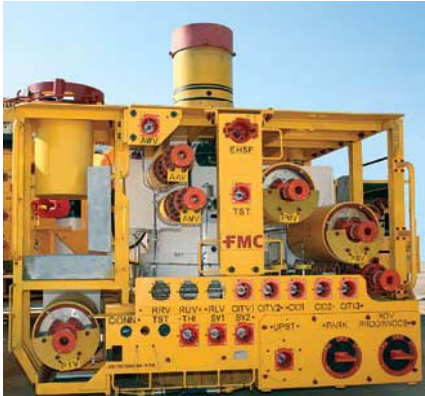
Figure 1.b 15K Enhanced Horizontal Tree (EHXT)[FMC,2009]
