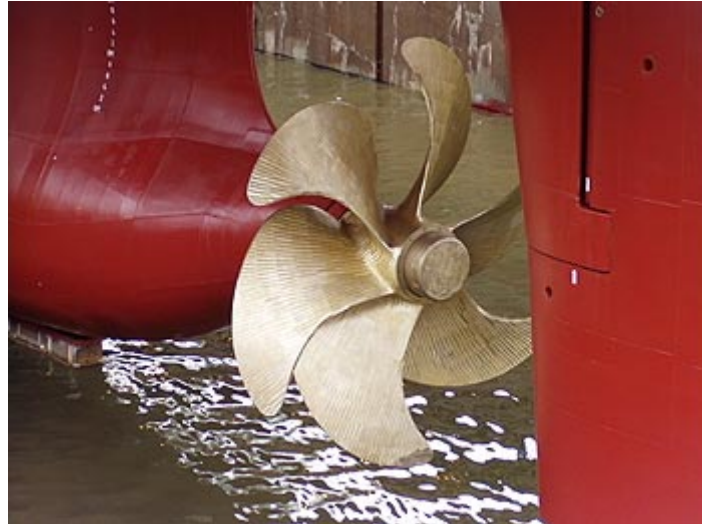
Figure 6.4. The engine is linked to a fixed pitch skew propeller (FPP). (Ref. - http://www.ship-technology.com/projects/manukai_maunawili/images/image5.jpg&imgrefurl )
