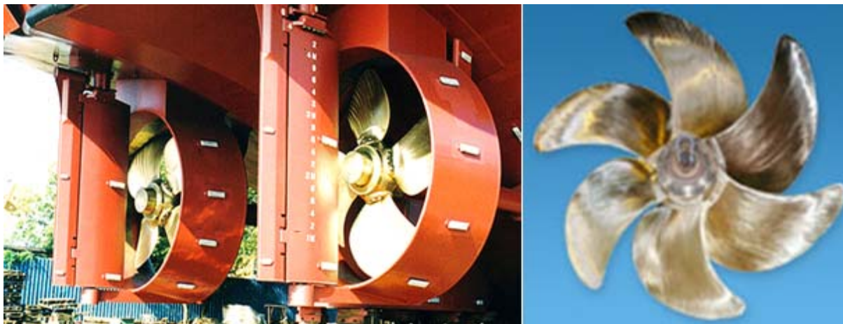
Figure 6.3. An example of a ship with fixed pitch propeller (FPP). (Ref. - http://www.wartsila.com/ ).
