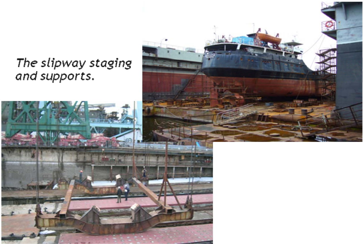
Figure 7.9. The outfitting quays, the slipway supports and the cranes of the plant.
