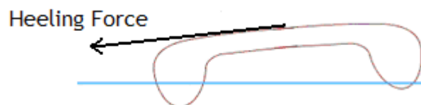
Figure 1.2. Heeling Force acting on a Catamaran.
