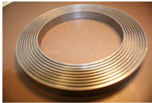
Figure 3-15 Photograph of flame gap surface CH-8.2.3, with eight crosswise grooves with width:2.0 mm and depth: 3.0 mm, investigated in experiments in the PCFA
