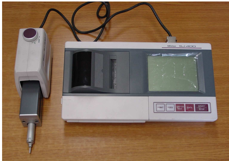
Mitutoyo SJ-400 - Apparatus used to measure surface roughness
