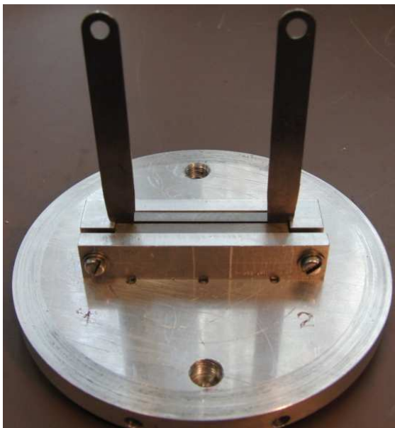
Figure A-2.5a Photograph of the upper part of the flame gap in the PRSA, with distance "shims" placed, the gap is fastened with a small torque applied on the screws seen in the photograph
