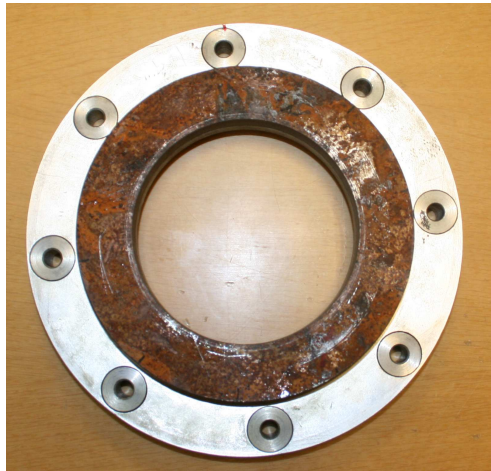
Figure 3-13 Photograph of the sandblasted flame gap surface examined in the PCFA. From (Opsvik 2010).
