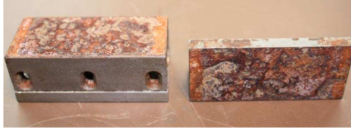
Figure 3-30 Photograph of rusted gap surface 2, examined in the PRSA
