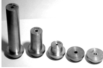
Figure 2-23 Various length of nozzles tested. From left; 100 mm, 50 mm, 25 mm, 12.5 mm all smooth nozzles, outermost right is threaded nozzles. From (Einarsen 2001).
