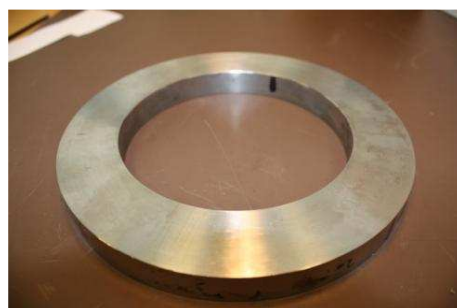
Figure 3-18 Photograph of the undamaged slit used in the experiments in the PCFA
