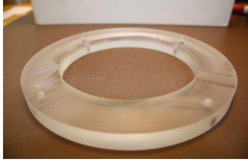
Figure 3-14 Photograph of Plexiglas flame gap surface examined in experiments in the PCFA
