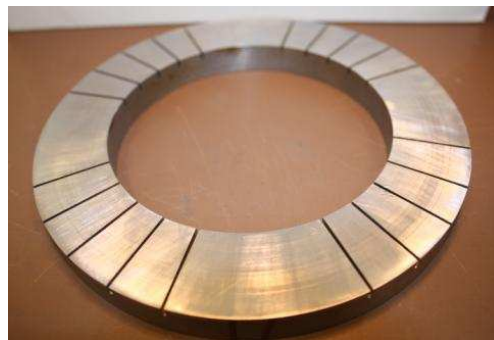
Figure 3-19 Photograph of the CV-20.1.4 flame gap surface, with twenty lengthwise grooves with width: 1.0 mm and depth: 4.0 mm, investigated in experiments in the MPCFA
