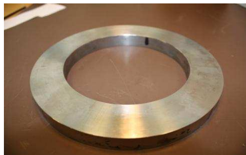
Figure 3-10 Photograph of the undamaged flame gap surface examined in the PCFA
