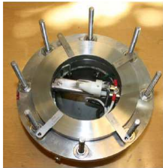
Figure 3-7 Photograph of apparatus flange, (flame gap) with the calibration shims in correct position. From (Opsvik 2010)
