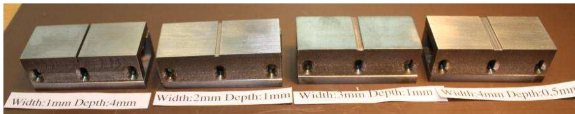
Figure 3-35 Photograph of five slits with different width and depth of the grooves on the gap surface that perforates the slit in the flow direction (lengthwise). Width and depth of grooves on slits, from left to right: Slit 1: width: 1 mm, depth: 4 mm. Slit 2: width 2 mm, depth: 1 mm. Slit 3: width: 3 mm, depth: 1 mm. Slit 4: width 4 mm, depth: 0,5 mm.
