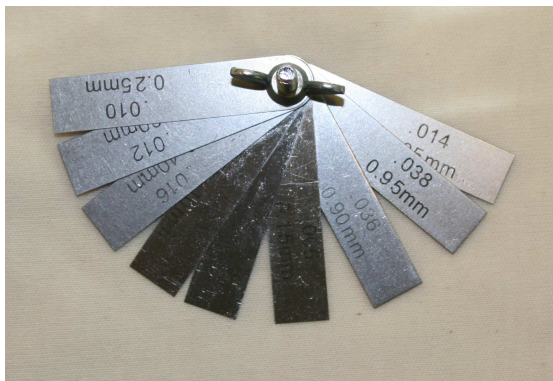
Figure A-2.3 Distance plates used to adjust the gap between the flame paths
