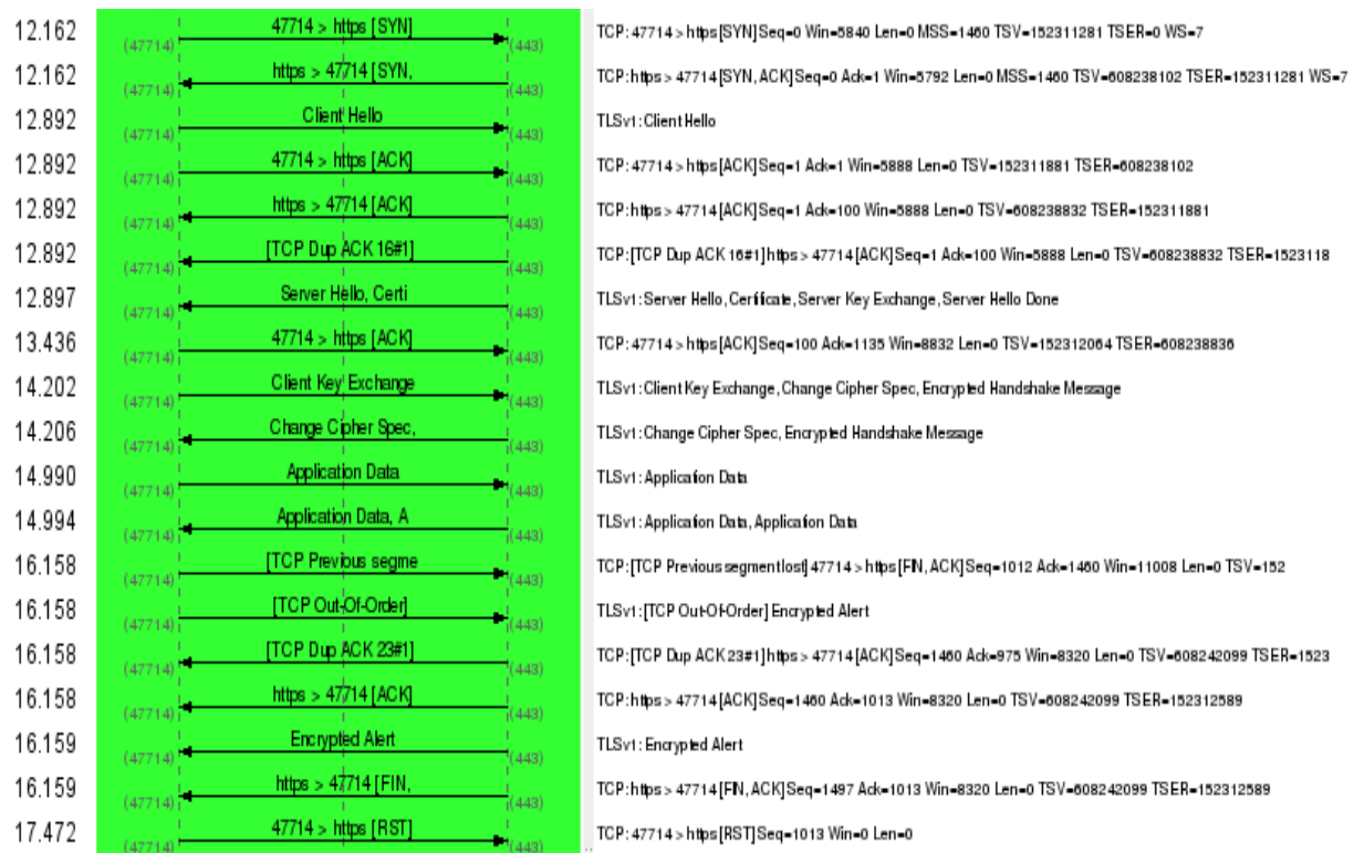
Figure 6-15: Flow graph of the TCP packets from the user agent to an escrow agent
