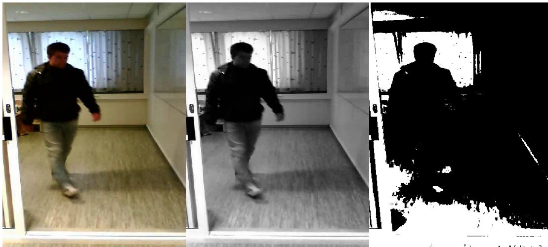
Figure 2.4: Application of Otsu: From left to right; original, gray scale and Otsu applied.
