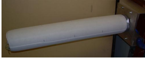
Fig. 6 Setup of inflatable boom attached at base plate.
