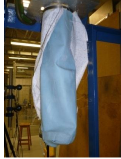
Fig. 3 Over pressurisation failure at 165 \text{ kNm}^{-2} of a 50 mm radius inflatable fabric boom.
