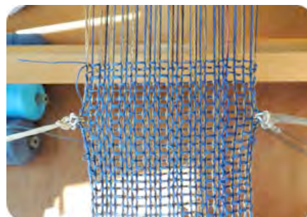
7. temple set-up to retain width of sample
