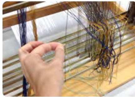
2. Doup ready to draw in twisting thread
