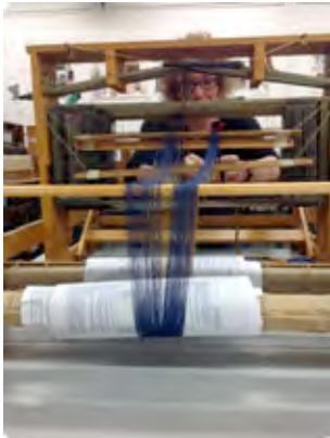
1. Warping up the loom
