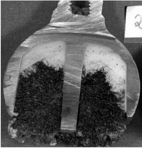
Fig. 5 Low-viscosity cement: incomplete seating
