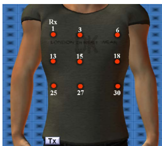
Fig. 9. Location of transmitter and receiver for on-body measurements using wireless sensor nodes at each carrier frequency.
