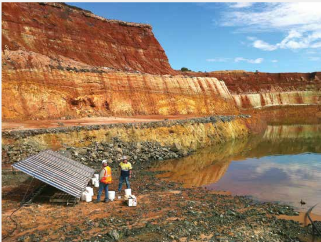
Caption: Pilot testing of pit water for a Gold mine in WA. Starting Total Dissolved Solids was 160,000 ppm (over four times that of seawater) and once treated by the Carocell unit was 0-3 ppm.
