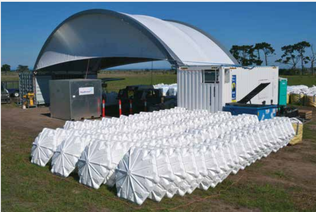
Caption: On-site Aqua Armour™ assembly system
