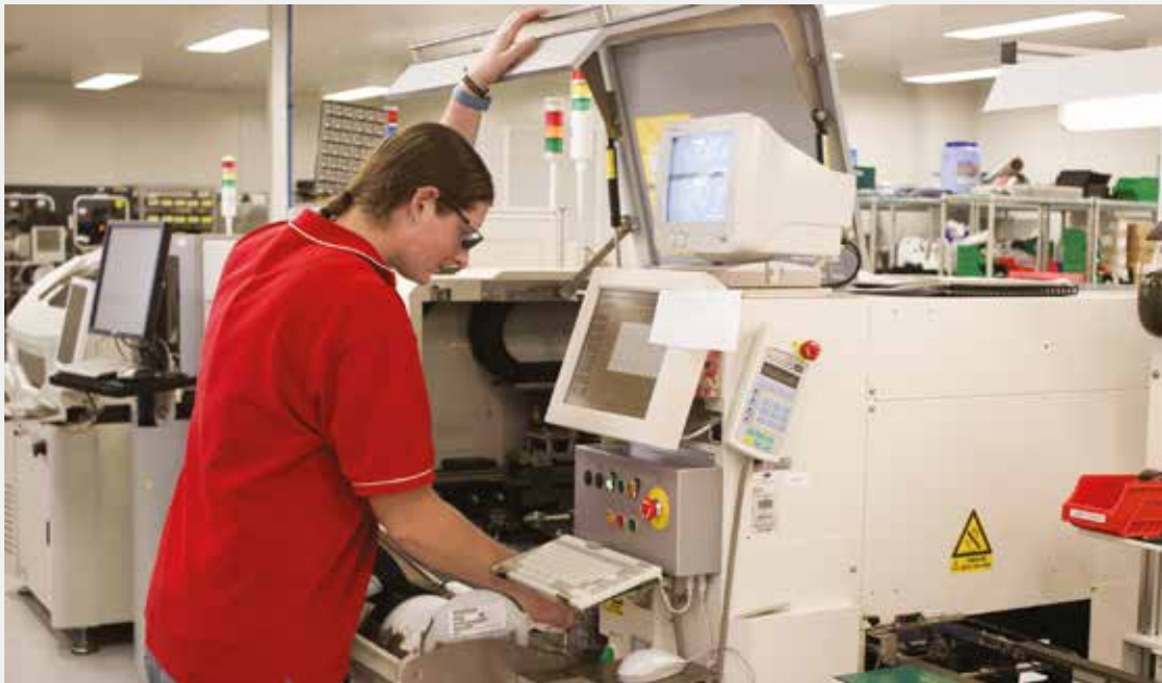
Caption: Operator using the pick and place machine
