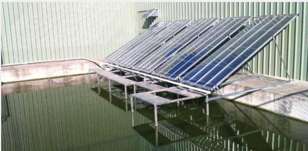
Caption: Carocell units processing waste wash down water from tractors and spraying equipment at a vegetable farm in Victoria. Image provided by F Cubed Australia.
