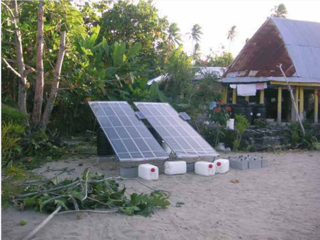
Caption: Resolving the daily canoe trip to another island to collect fresh water, the Lions Club of Apia contributed 40 Carocell units to the community of Manono Island in Samoa to process seawater into drinking water. Images provided by F Cubed Australia.
