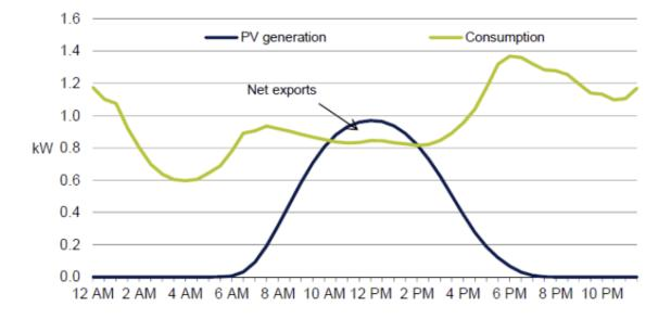
NSW average electricity consumption and PV generation over 24 hour period. Source: <u>Estimating a fair and</u> <u>reasonable solar feed-in tariff for Queensland</u>. The green line shows the average consumption for a household, the blue line the average electricity generated by PV panels. When the blue line exceeds the green the household will be using self-generated electricity instead of drawing from the grid, if on a net metering system.
