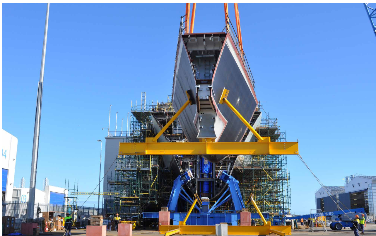
Consolidation of final keel block for first Air Warfare Destroyer. Photo courtesy of the Department of Defence.
