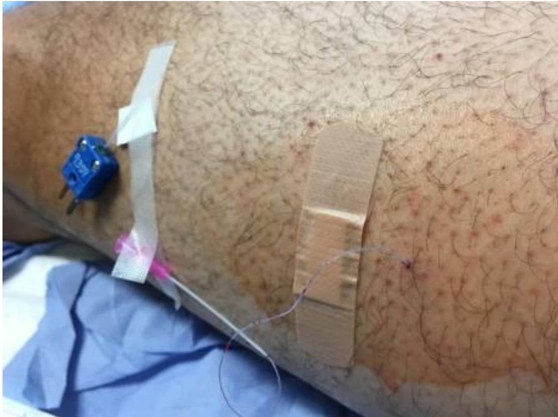
Figure 16: One thermocouple inserted into vastus lateralis showing flexible catheter (pink) threaded over the thermocouple towards the thermocouple 'head' away from the insertion site. The thermocouple head was later plugged into an extension cable and connected to the digital monitor once fully instrumented. A second thermocouple was subsequently inserted as described above (section 6.2.3), and both insertion sites were secured with sterile tegaderm prior to initiation of both treatments.
