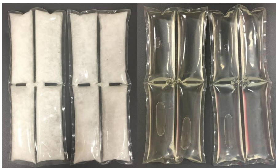
Figure 6: Two Glacier Tek PCM packs in the frozen state (left), and in their melted state (right).
