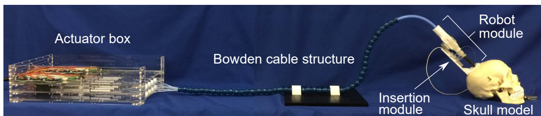
Figure 6.3: The complete cable-driven remotely-actuated neurosurgical robotic system
