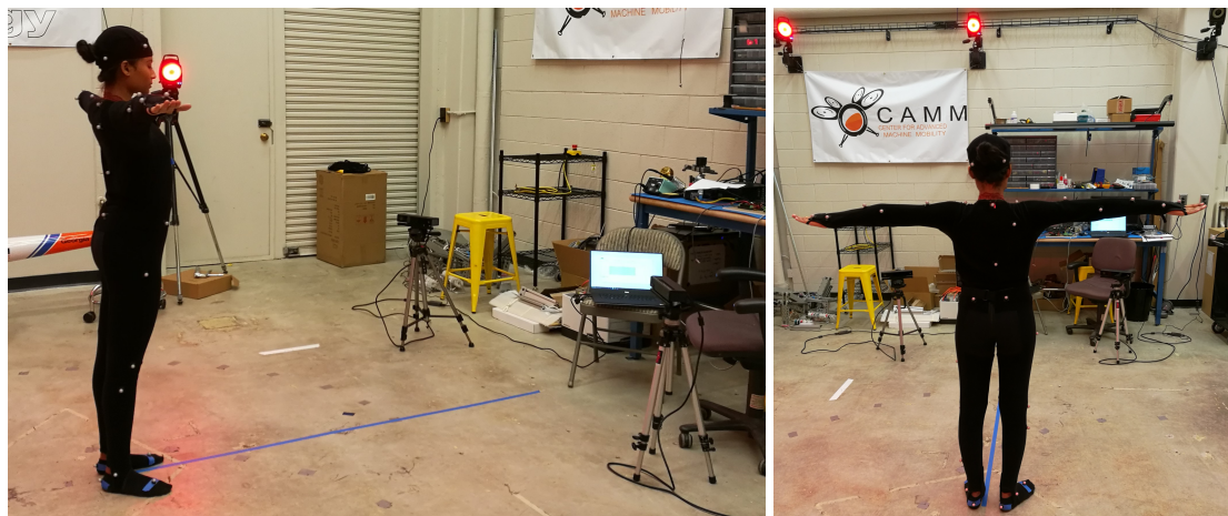
Figure 5.5: Test Subject Standing in T-Pose and Dual-Kinect Test Setup
