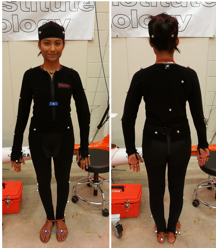
Figure 5.6: Marker Placement for Full Body Plug-in-Gait Model on Test Subject
