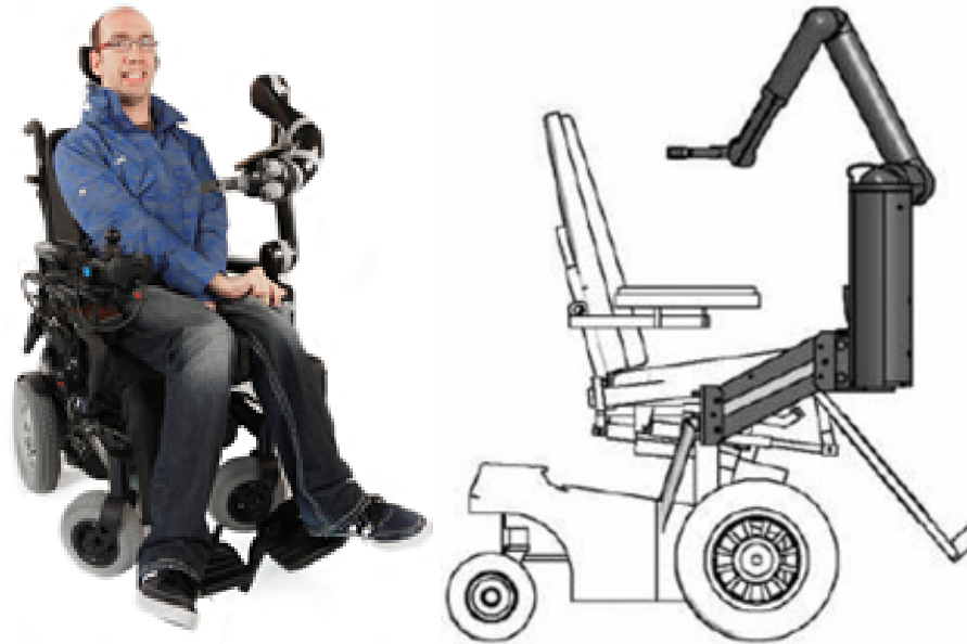
Figure 2.2: Left: JACO robotic arm mounted on a powered wheelchair copied from [117]. Right: UCF-MANUS copied from [116].
