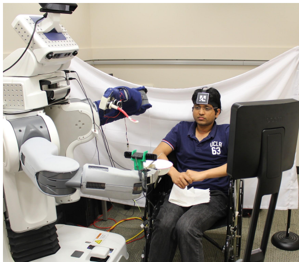
Figure 5.15: Our system feeding yogurt to an able-bodied person. A person with quadriplegia commanded the system remotely.
