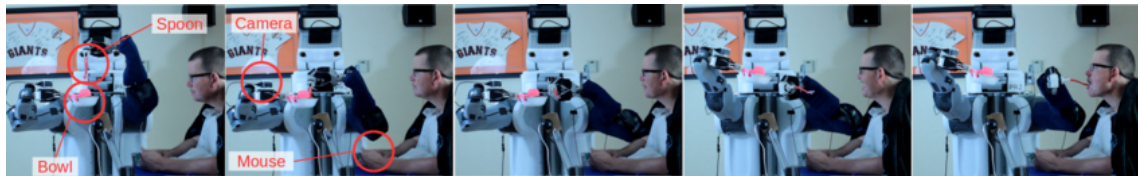
Figure 4.7: An image sequence of the entire scooping and feeding process with Henry Evans, a person with quadriplegia, in the living room of his home.
