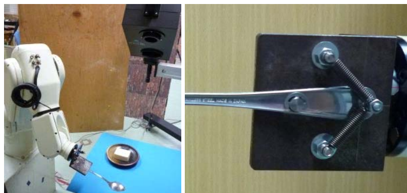
Figure 2.6: A meal support system and its spring-attached spoon copied from [137]
