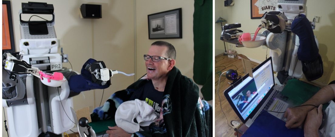
Figure 5.16: Left Henry Evans, a person with severe quadriplegia, successfully used our robot-assisted feeding system in his home to feed himself while our execution monitor was running. Right A capture of Henry’s head tracker and one-button mouse.
