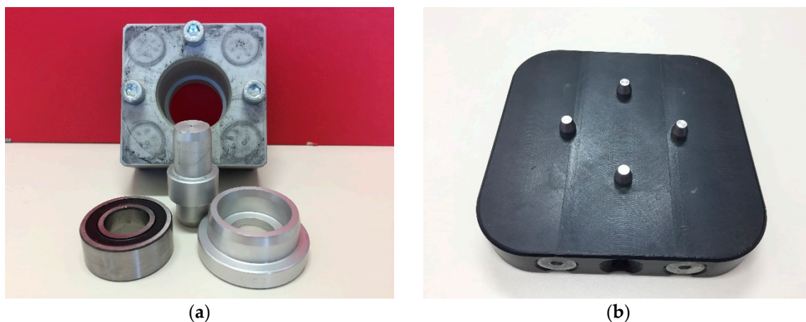
Figure 1. Detail of pieces managed in the FMS: (a) Constituent elements of the turning mechanism; (b) Transport pallet.
