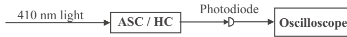
Figure 4.5: Experimental setup of absorption spectroscopy with 410 nm light on the hollow cathode (HC) and the all-sapphire cell (ASC), respectively. In the experiments, the discharge current of the hollow cathode is 10 mA and the temperature of the sapphire cell is 630 °C.
