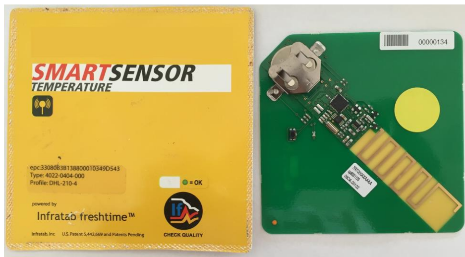
Abb. 21: SmartSensor Temperature (eigene Abb., Fa. Infratab, Oxnard, USA 2009).
