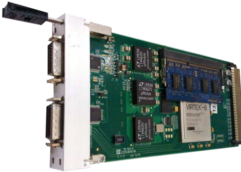
Figure 3.22: DHH prototype. Based on Virtex-6 FPGA, version insertable in ATCA Module.
