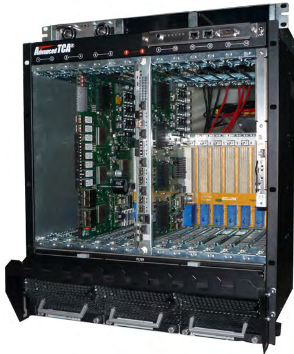
Figure 3.23: The ATCA shelf with two Compute Nodes installed [45].
