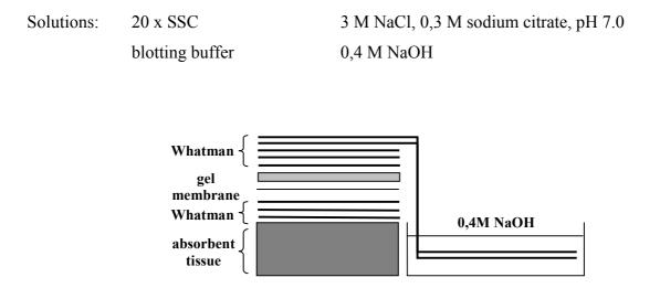
Figure B2: Assembly used for Southern transfer
