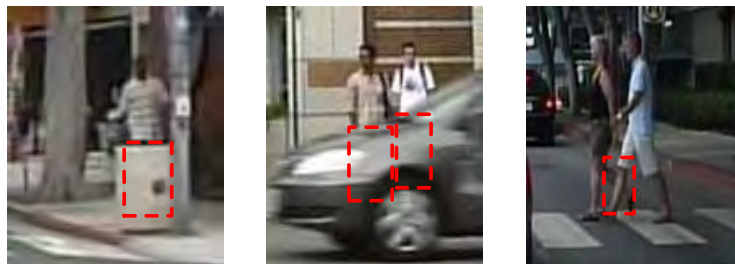
Figure 3.10: Three examples of occlusions happen at lower body. Example images are from the Caltech pedestrian data set, and red dashed bounding boxes are used to indicate the occluded body parts. In the given examples, occlusions are caused by a dustbin, a moving car and another walking-by pedestrian, respectively.
