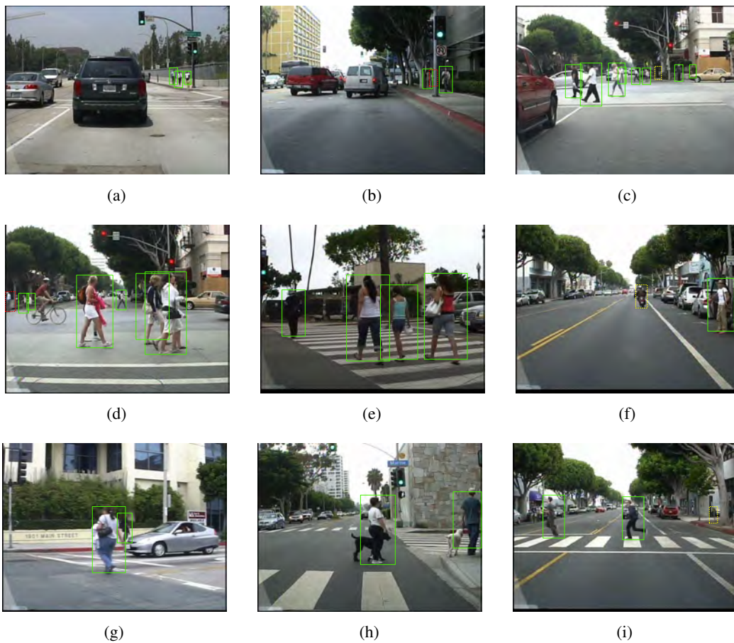
Figure 3.11: Detection examples of our detector under different scenarios from the Caltech pedestrian data set. Green solid bounding boxes, yellow dotted bounding boxes and red dotted bounding boxes indicate true positive, false positive and false negative (missed) results, respectively. (a) Small scale pedestrians walking along the street. (b) One missed pedestrian due to heavy occlusion (> 70%). (c) Complex scenario at one intersection with one false positive occurring at one tree. (d) Pedestrians with occlusions. (e) Multiple pedestrians walking across the street. (f) One motorcyclist falsely detected as a pedestrian. (g) One pedestrian of low contrast. (h) Pedestrians with pets. (i) One traffic sign falsely detected as a pedestrian.
