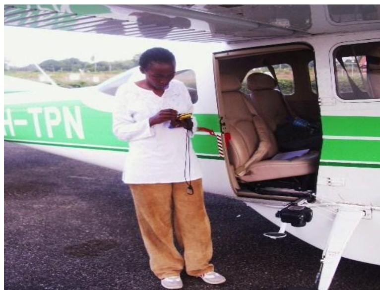
Figure 3.13: Camera setting, plane doors removed and a camera mounted outside
