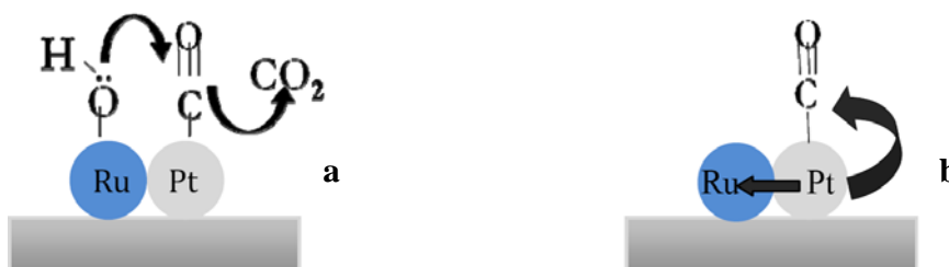
Figure 1-10: The mechanisms of Ru effect on the electrooxidation of CO at Pt surface a) Bifunctional effect and b) Ligand field effect (electronic effect).
