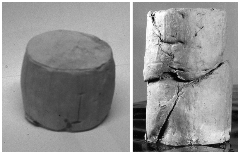
(a) Uniform shear for plastic Tertiary clay from the field site Melbtal.
