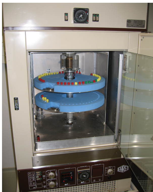
Figure 2.3: Multi-Sample Incubator Centrifuge (MuSIC) at DLR.
