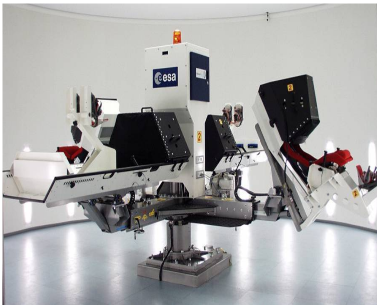
Figure 2.4: Short-Arm Human Centrifuge at DLR in Cologne (Source: ESA).
