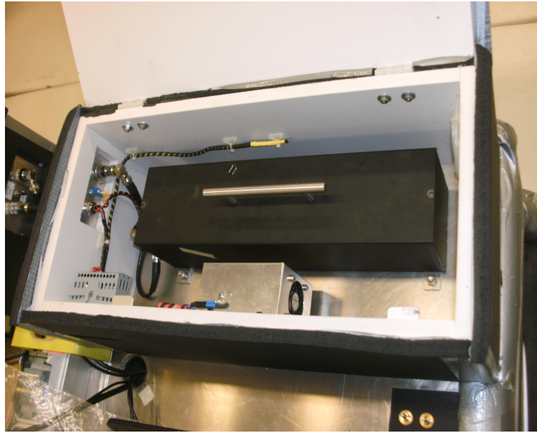
Figure 2.7: Forex heating box with PMT-Clinostat (black box). Design: Kai Wasser (DLR, Cologne)
