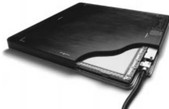
Fig. 3.8: Flat-panel active-matrix direct-conversion X-ray imager using an amorphous selenium conversion layer with an imaging area of 36 x 43 cm (courtesy of Hologic Inc.) [13].
