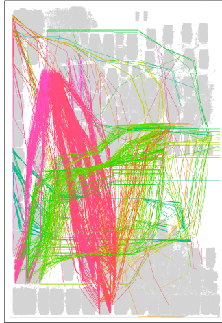
Figure 7.6: All repeater chains longer than 4 mm on a large design. Distributing the chains more evenly can give us less congestion while preserving the timing.
