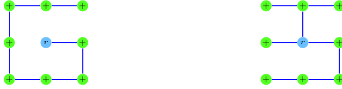
Figure 5.2: Two topologies with the same shortest possible length but different timing behaviour. While all sinks are reached within 4 segments on the right side, it takes up to 8 segments to the furthest sink on the left side.
