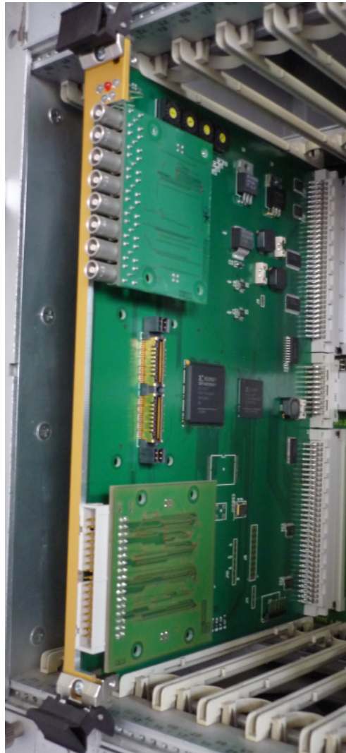
Figure 59: VME FPGA mainboard (VFB) with NIM and ECL mezzanine plugged on.
