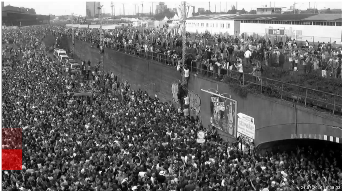
FIGURE 4.21: Detection of Crowd Turbulences. Camera 13 which monitored the main entry ramp shows short sequences of shock waves that are propagated. We automatically detect regions of high pressure which are colored red in the above Figure. Note that the saturation of the alarming cells have been increased for the sake of visibility.
