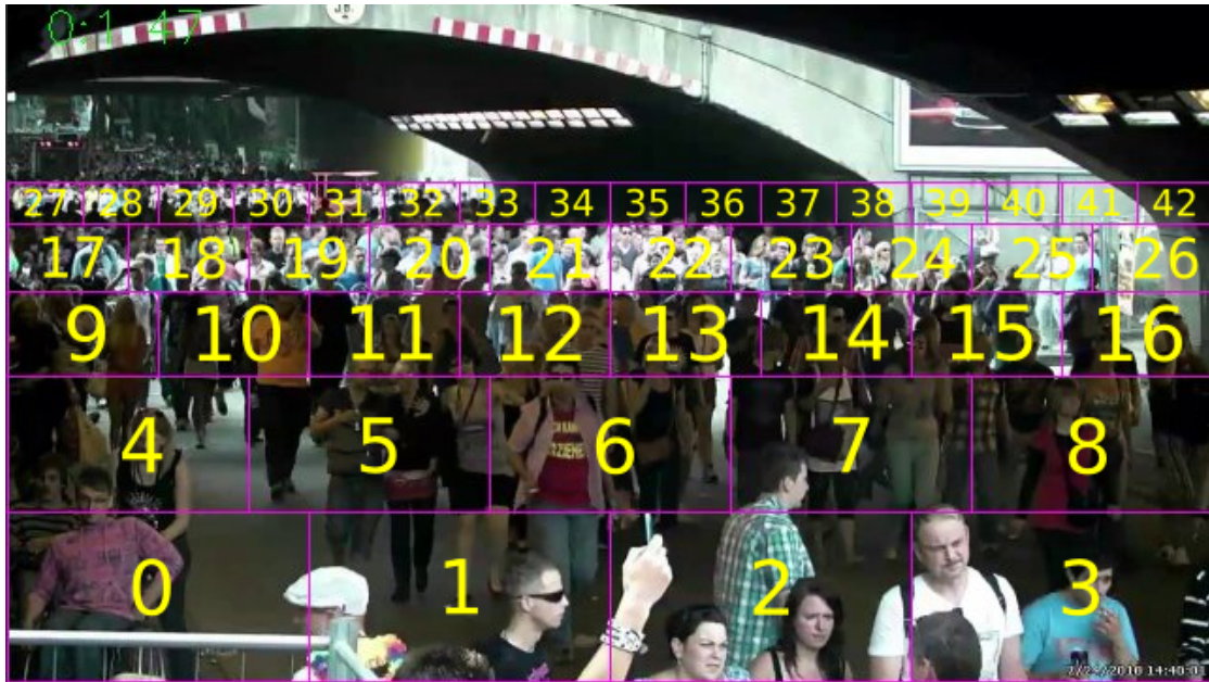
FIGURE 3.7: Superposition of a grid over the video frames where grid cells towards the back of the scene are smaller accounting for perspective distortions.
