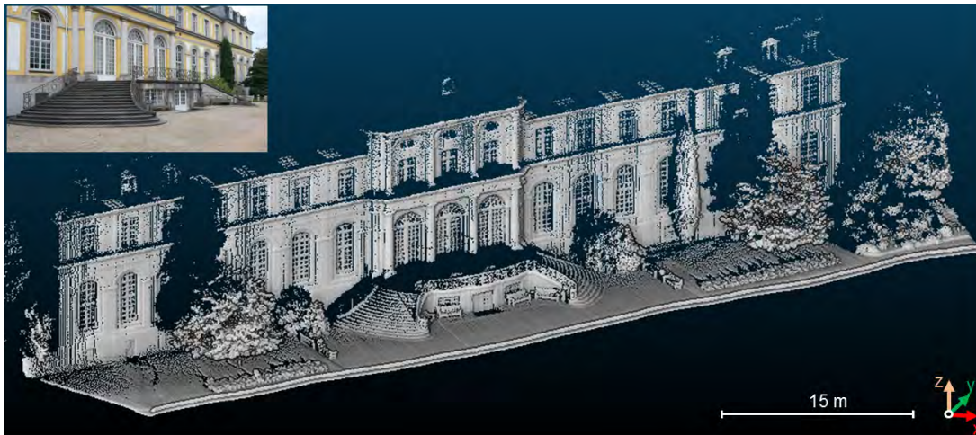
FIG. 13. Directly georeferenced point cloud of a building. The points were generated in real-time without any post processing.
