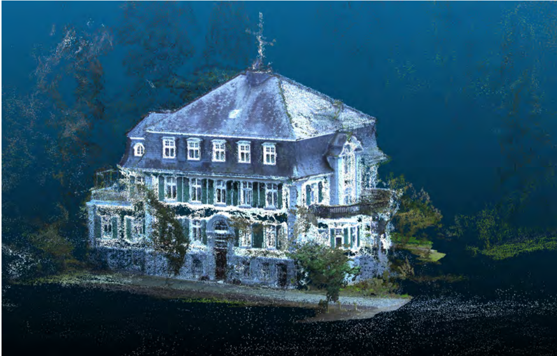
FIG. 10. Georeferenced point cloud of a building and surrounding vegetation. The cloud is actually the union of three clouds generated from images from three different flights.
