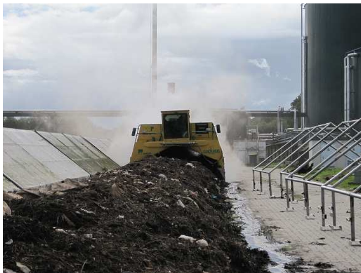
Figure 1.4: Triangular composting window is turned by a special windrow turner
