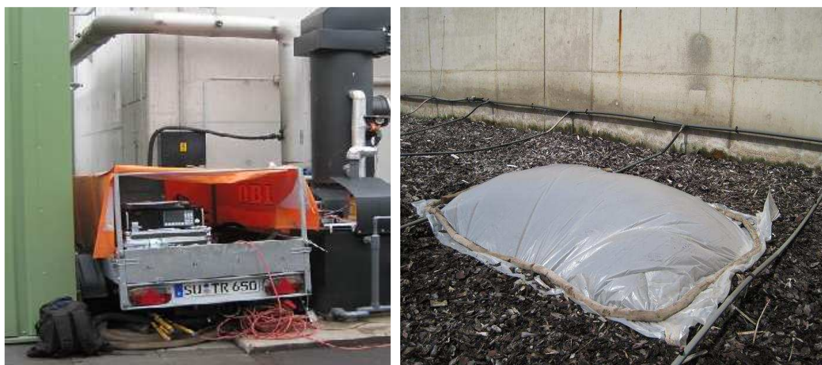
Figure 2.15: Left: Sampling of gases at before biofilter and measuring equipments. Right: Foil covers on a biofilter for \text{CH}_4 , \text{N}_2\text{O} and \text{NH}_3 concentration measurements
