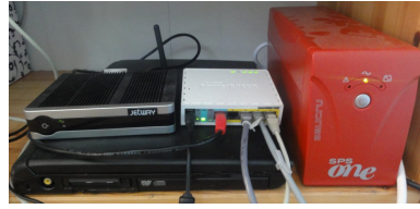
Figure 4: Indoor hardware of a community network node with router, server and cloud resource
