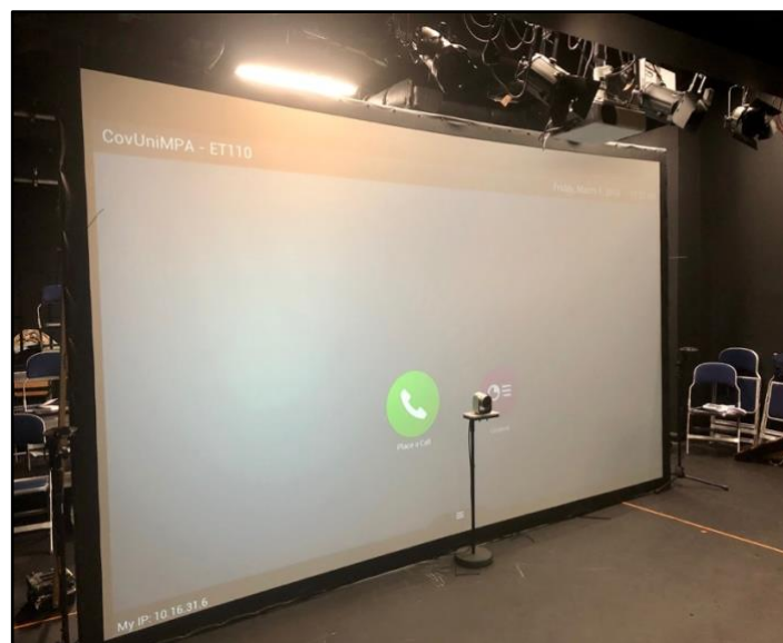
Figure 3: View of the rear projection screen during set up. The Polycom camera is placed just above average waist height using a thin microphone stand, the screen is flush to the floor and the directional microphones are located either side of the screen
