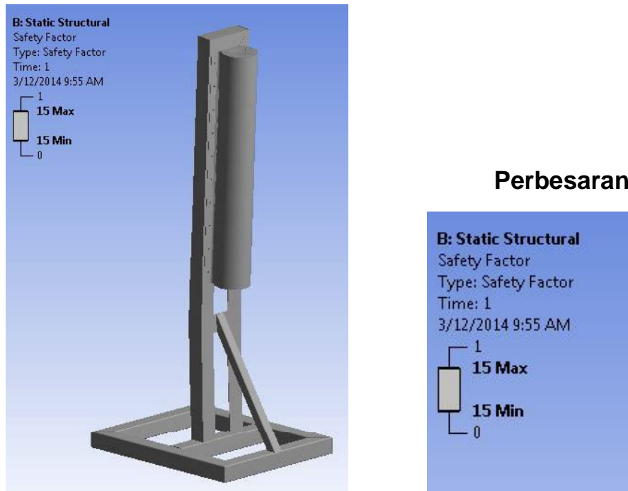
Gambar 6. Hasil analisis safety factor
