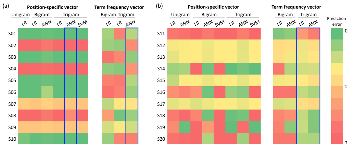
Figure 3.4. Absolute prediction error heat map of (a) initial models and (b) 1 st retrained models vs. experimentally identified sequences. Total prediction errors were calculated using eq (3.1) then normalized by twice the number of instances ( = 2 \times 10 ): For the initial models with psv , values are 0.4, 0.4, 0.395, 0.4, 0.38, and 0.4 for unigram LR, bigram LR and ANN, trigram LR, ANN, and SVM, respectively. For the initial models with tfv , values are 0.479, 0.564, and 0.423 for bigram LR, trigram LR and ANN, respectively. For the 1 st retrained models with psv , values are 0.638, 0.605, 0.763, 0.394, 0.8, 0.42, 0.405, and 0.6 for unigram LR and ANN, bigram LR, ANN, and SVM, trigram LR, ANN, and SVM, respectively. For the 1 st retrained models with tfv , values are 0.6, 0.434, 0.317, and 0.324 for bigram LR and ANN and trigram LR and ANN, respectively. Overall, ANN for both trigram psv and tfv of initial models and LR and ANN with trigram tfv of 1 st retrained models showed the best performance (highlighted with blue box).
