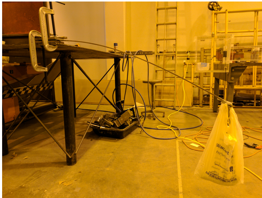
Figure 12: The cantilever beam test setup with a four pound loading on the end.
