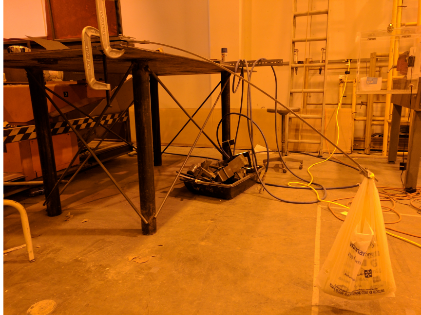
Figure 13: The cantilever beam test setup with a six pound loading on the end.
