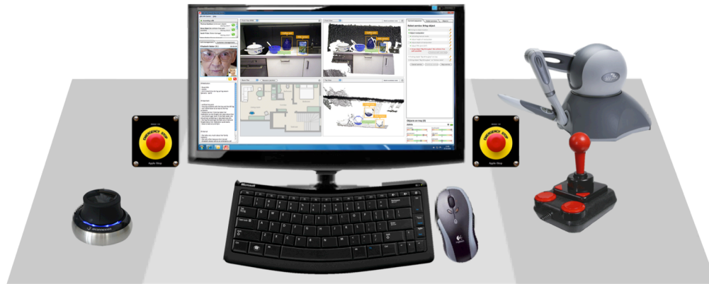
Figure 10. Workstation hardware concept for 24-hour teleassistance service staff consisting of monitor, keyboard, mouse, two emergency stop buttons, joystick, 3Dconnexion SpaceNavigator 3D mouse (front left), and Sensable Phantom stylus-based 3D haptic manipulation device (back right)
