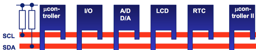
Figure 2.2: I2C typical topology. Extracted from [24].
