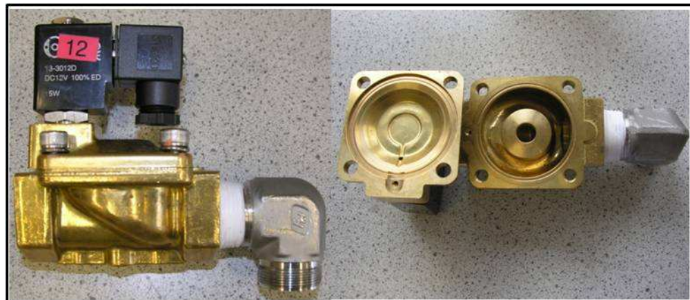
Figure 6.6 The specific structure of the solenoid valve
