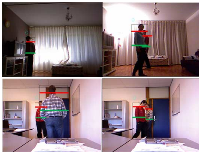
Fig. 6. Head region detection at different locations, where red line indicates the neck position.
