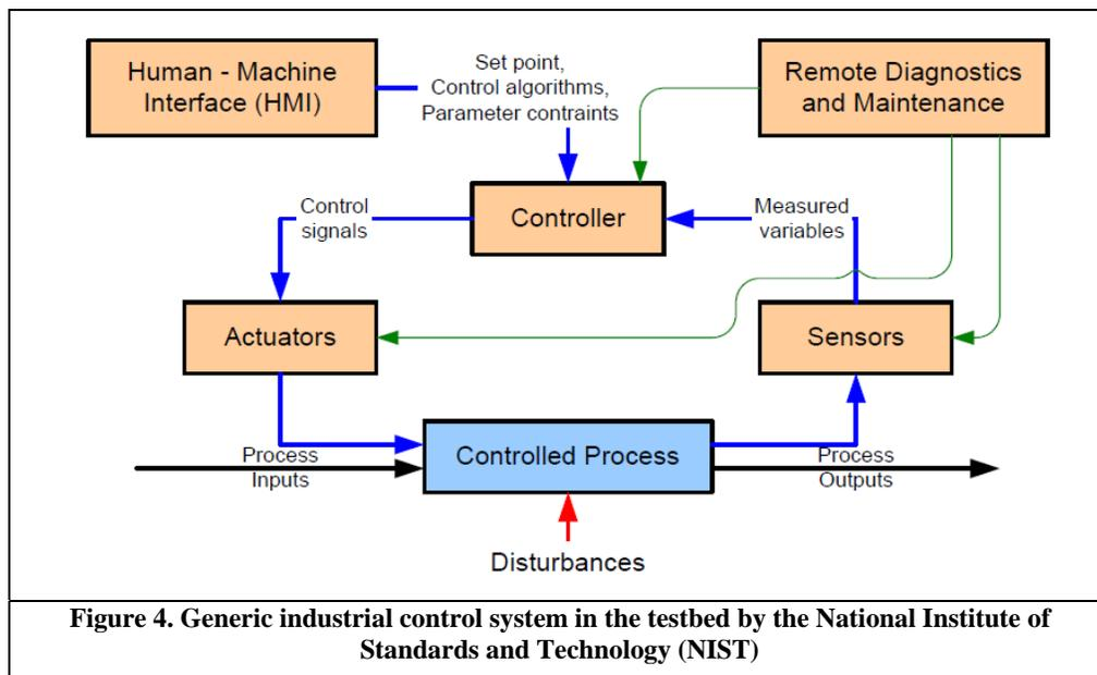
Figure 4. Generic industrial control system in the testbed by the National Institute of Standards and Technology (NIST)
