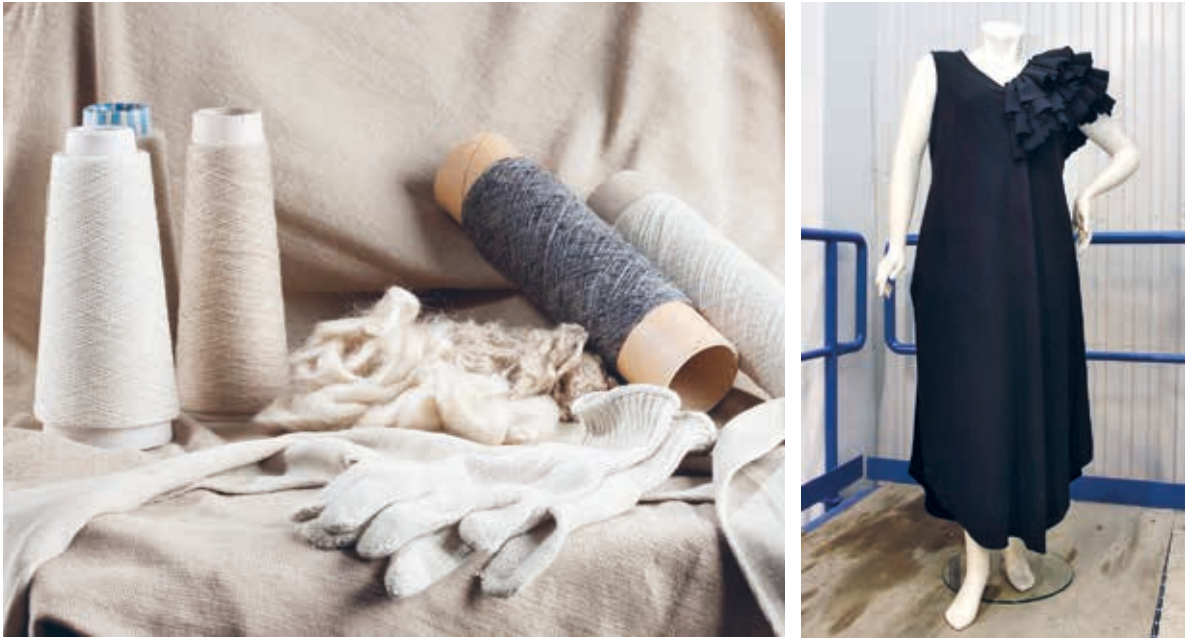
Figure 4. Carbamate fibers made from textile waste and products made from this material (photos by VTT).
